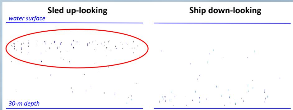
A comparison between the echograms, or hydroacoustic readouts, of the ship-based down-looking echosounder (right) and sled-based up-looking echosounder (left) along a 15-minute transect in August 2018 on Lake Superior. Blue blips are individual fish measured within the uppermost 30 meters of the water column. Image credit: USGS
